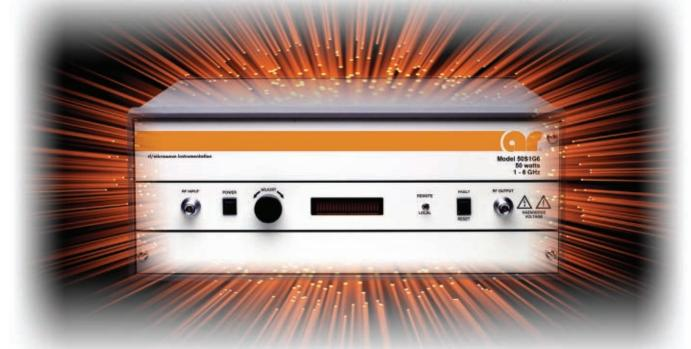
Now you can finally purchase the amplifier products you need to fulfill your wideband EMC and wireless applications in one amplifier. AR's new amplifiers offer 15 to 50 watt Class A linear power versions over an instantaneous BW from 1 to 6 GHz with very low harmonic distortion for your demanding requirements. These units can be driven with as little as 1 mW and provide excellent flatness across the operating frequency band in addition to excellent noise figure.
