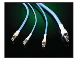
Times Microwave TF4 dielectric material is the key ingredient, making our <u>PhaseTrack products the best choice for phase critical</u> interconnect applications. PhaseTrack cable dielectric was developed to eliminate the "PTFE knee" in the phase/temperature performance of cables for phase-critical applications.
