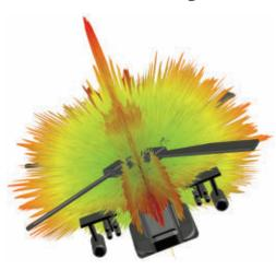
RCS & Surface Current Simulation of a Helicopter
