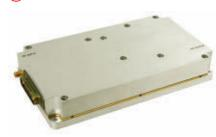
Empower model BBM2E3KLP is a 20 to 520 MHz amplifier that is guaranteed to deliver 125 W output power and related RF performance under all specified temperature and environmental conditions. The amplifier module is  $7" \times 4" \times 1.5"$ . This amplifier is suitable for broadband jamming and high power linear applications in the UHF/VHF bands. This module utilizes high power LDMOS transistors and also features built in control and monitoring, with protection functions.
