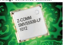
The SMV5550B-LF, a high performance VCO, generates frequencies between 5000 and 6000 MHz, covering the 1000 MHz bandwidth within 0 to 10 V of control. Though the device covers a broad spectrum of bandwidth, the SMV5550B-LF comes in a compact package covering an area less than .10 sq. inches while exhibiting phase noise performance of -80 dBc/ Hz, typically, at 10 kHz from the carrier. It delivers  $3 \pm 3$  dBm into a 50  $\Omega$  load with a nominal 5 V supply and drawing typically 24 mA.
