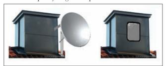
▲ Fig. 1 Parabolic reflector for a point to point microwave link, compared to small flat array for mm-wave.
