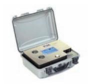
1800 is a full band unit for the 1800 band, applicable for GSM1800, LTE Band 3 and LTE Band 9. PIMPro is a ruggedized field tool, with a flexible touch screen and icon-driven user interface, which enables PIM testing to be done swiftly, efficiently and with confidence by the field technician.
