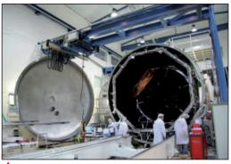
Fig. 1 Thermal vacuum chamber.
